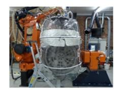
Manufacturing of titanium components for aeronautics by  ${f LMD-w}$
