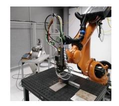
Manufacturing of graded components with a functionalised surface by **LMD-p**
