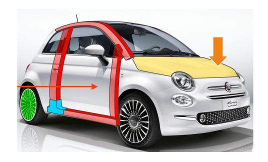
Cold reforming of external non-structural elements
